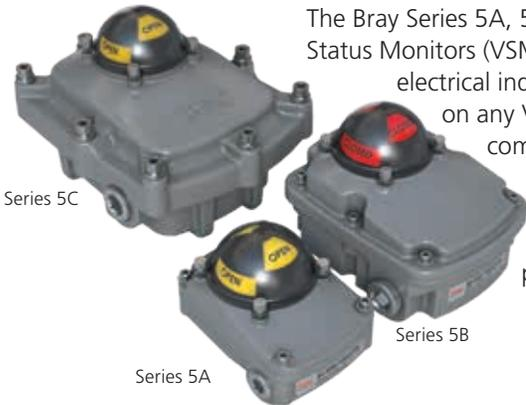
The Bray Series 5A, 5B and 5C Valve Status Monitors (VSM) provide visual and electrical indication of position on any VDI/VDE 3845 compliant quarter-turn device. Our solutions enable end users to better monitor their process no matter the conditions.
