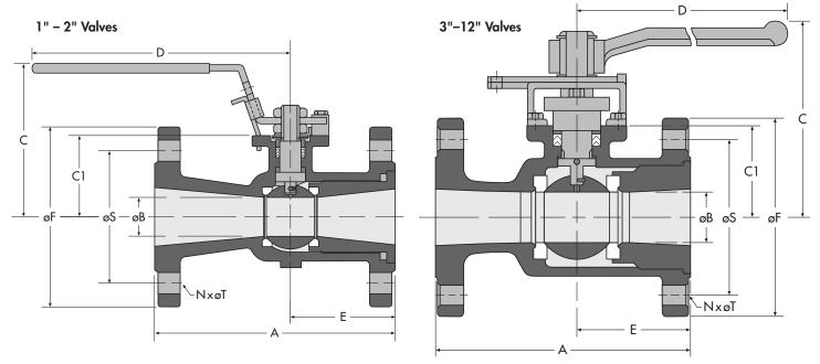
NOTE: Gear Operators are suggested on size 10" and 12" valves. NOTE: A trunnion-like Ball Support is included on size 12" valves.
