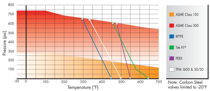
Carbon Steel valves limited to -20°F
